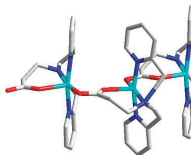
Fig. 7 Representation of the 1D coordination polymer of [\text{Cu}^{\text{II}}(\text{L}^{11})][\text{ClO}_4] \cdot 2\text{H}_2\text{O} ( 13 ).
